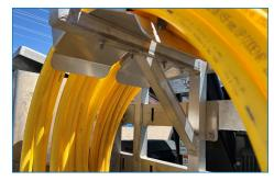
bought two poly holders, added a bracket to the top and bottom so it can hold both sizes. They also added an aluminum box on the bed to carry straps and hoses. These modifications gave Riddle more organization and productivity at the iob site.
